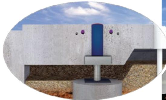
*Lifting mechanisms elevate the slab to create a protective void.*
