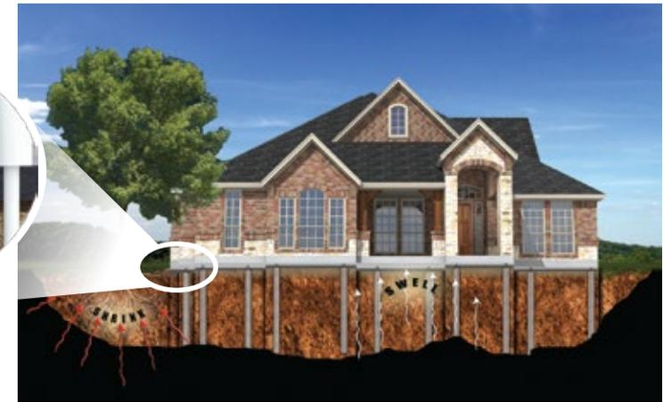
Designed to perform as a suspended slab, Tella Firma provides the strength of a pier-and-beam foundation system, yet is much more affordable and takes less time to install than most traditional suspended foundations.
